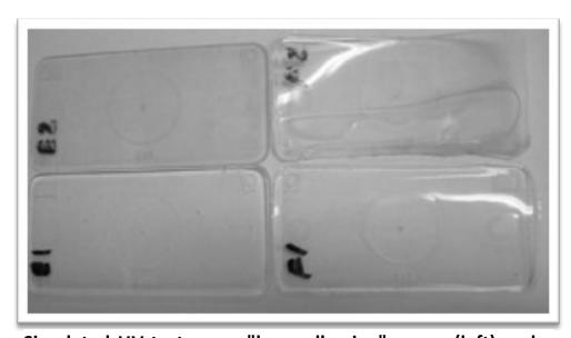
Simulated UV tests on a "low yellowing" epoxy (left) and a PU. The original samples are on the bottom, while the samples on top have been weathered for the equivalent of 2 years. Substantial yellowing can be seen in both!
