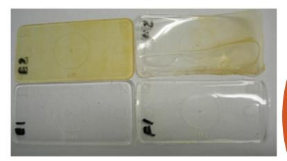
UV tests on a low-yellowing epoxy (left) and a PU show they both yellow.
