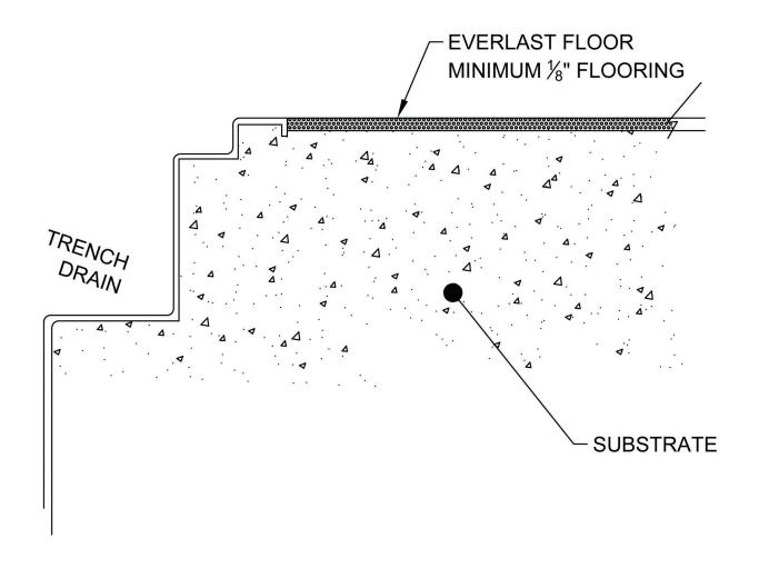
NOTE: TOP OF DRAIN TO BE LEVEL WITH OR LOWER THAN TOP OF SUBSTRATE.
