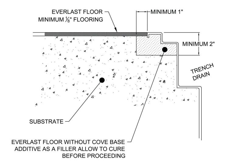
NOTE: TOP OF DRAIN TO BE LEVEL WITH OR NOT MORE THAN 1/8" HIGHER THAN SUBSTRATE.
