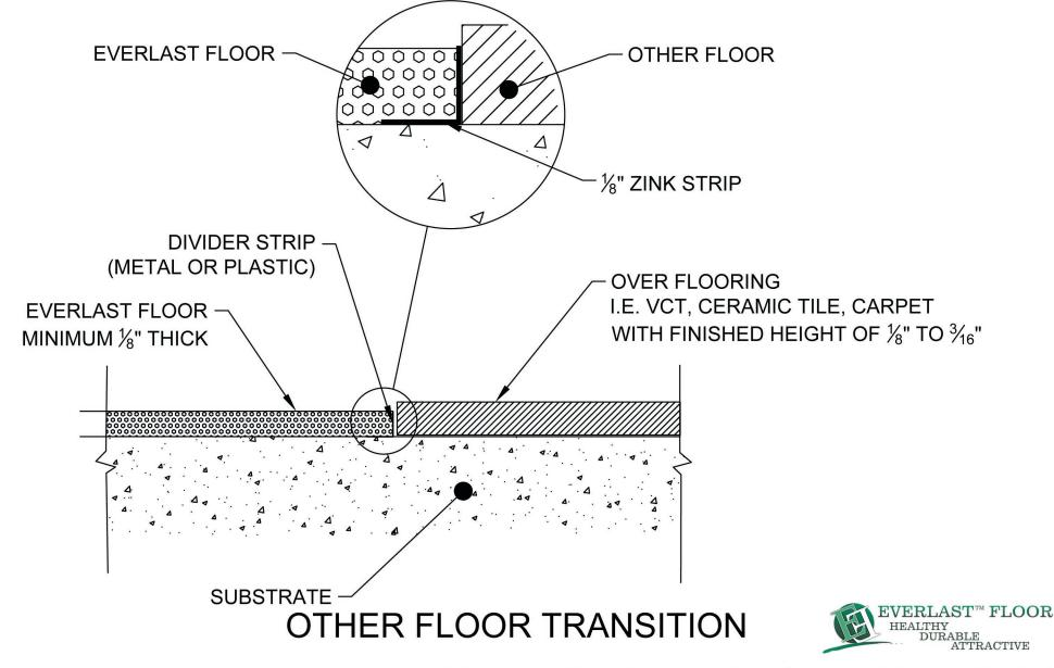
Finished transition of Everlast Floor (commercial epoxy flooring) to another floor finish of similar thickness
