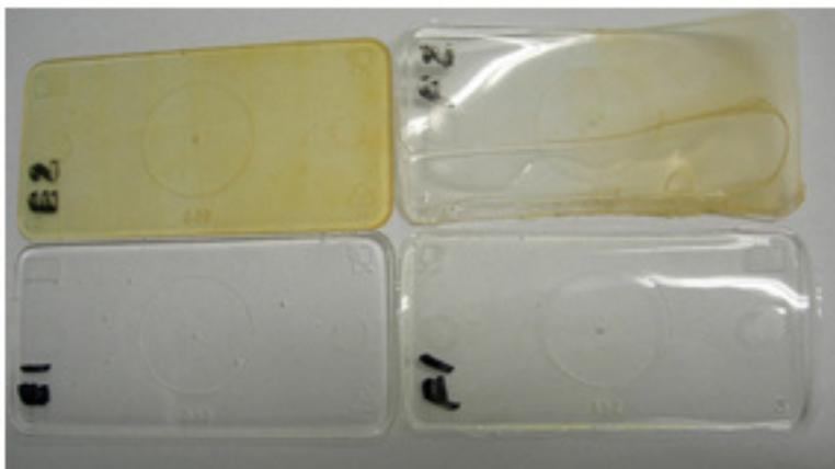
UV tests on a low-yellowing epoxy (left) and a PU show they both yellow.
